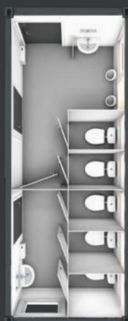
SA5 20' Damen/Herren WC-Container
